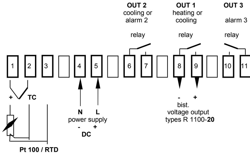
It is not permitted to connect the grounds of the sensor- and bist. voltage-outputs with each other.
